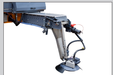
Long rear end for optimal centre of gravity positioning. Stainless spreading disc and funnel.
