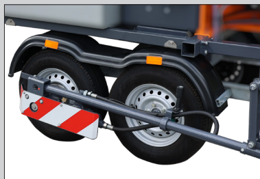
Can be powered by hub drive from the vehicle.
