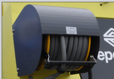
Optionally, hose drum can be mounted.
